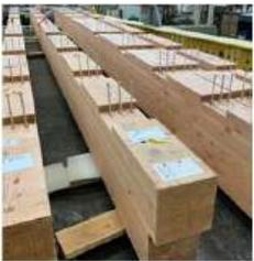
Glued laminated timber is characterized by high load-carrying capacity, dimensional stability and the ability to form the timber components into almost any shape.
